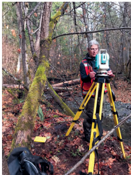
Florance Condos leveling the total station on Horse Creek on November 25, 2020. Florance is using the total station to collect accurate coordinates of the logs installed for the Horse Helicopter Wood Loading Project.
