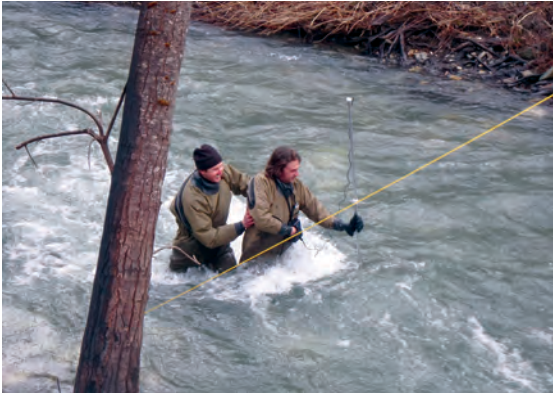
Jimmy Peterson gets some help from Tony Dennis taking discharge measurement on Horse Creek on February 27, 2017.
