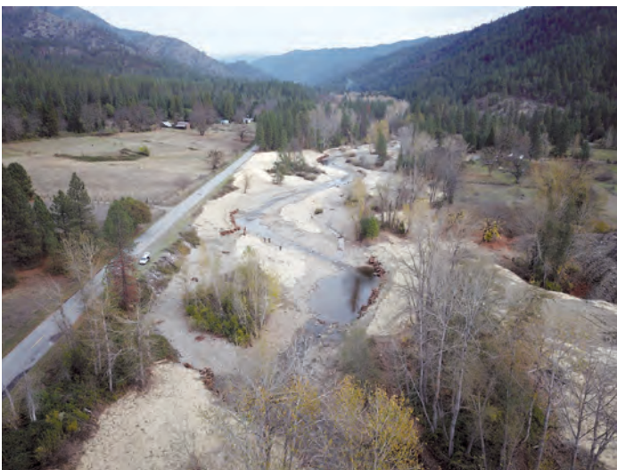
Apex jam installed for the Seiad Reconfiguration Project. This jam will help the constructed side channel functioning. Split channels, side channels, and alcoves all help diversify the stream habitat for aquatic organisms. Seiad Creek on April 7, 2018.
