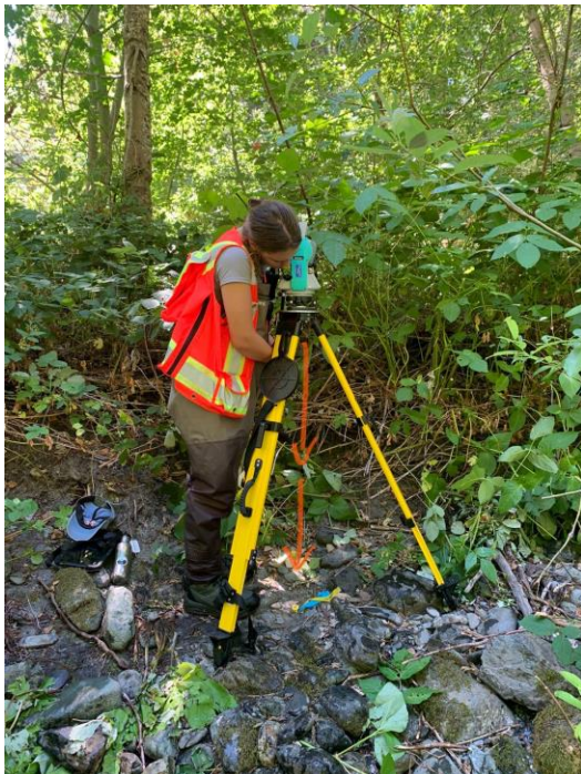
Looking through, aligning the Total Station with the Station point
