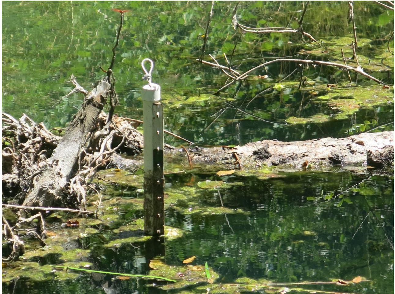
Photo: Water level logger well deployed in pool one of Durazo Pond. Photo was taken in July of 2016 and previous winter's high water mark can be seen on the pipe.
