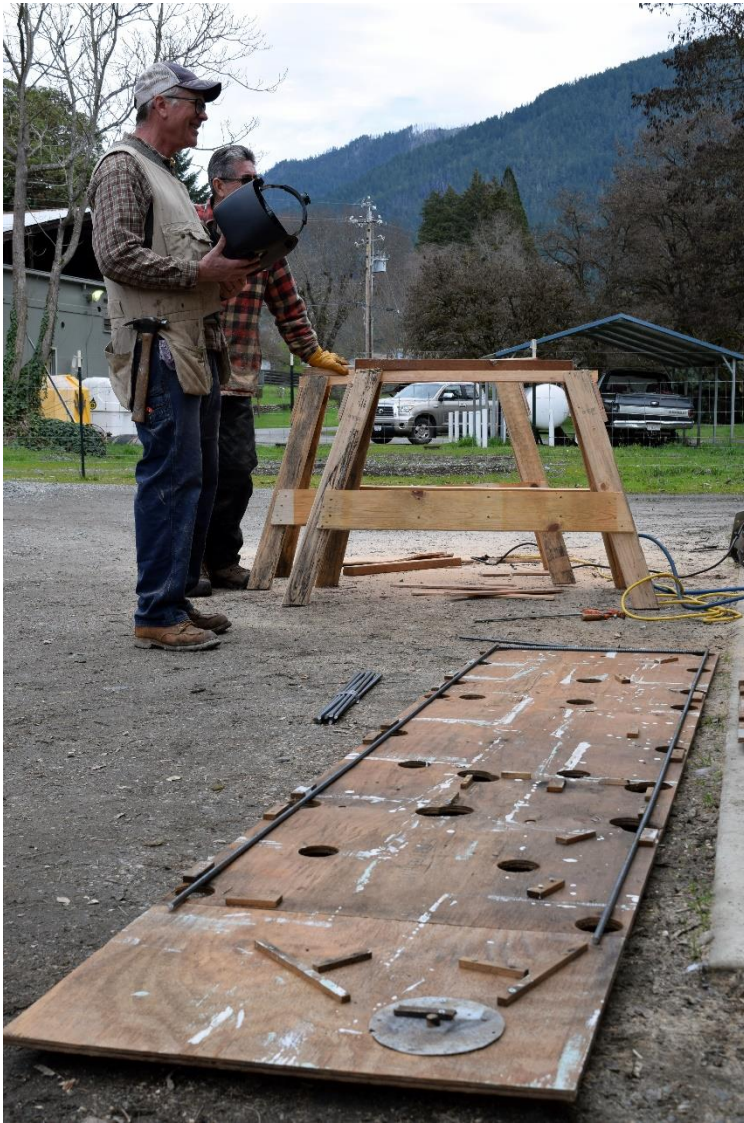
7. Wilson's template, used to weld the long side panels.
