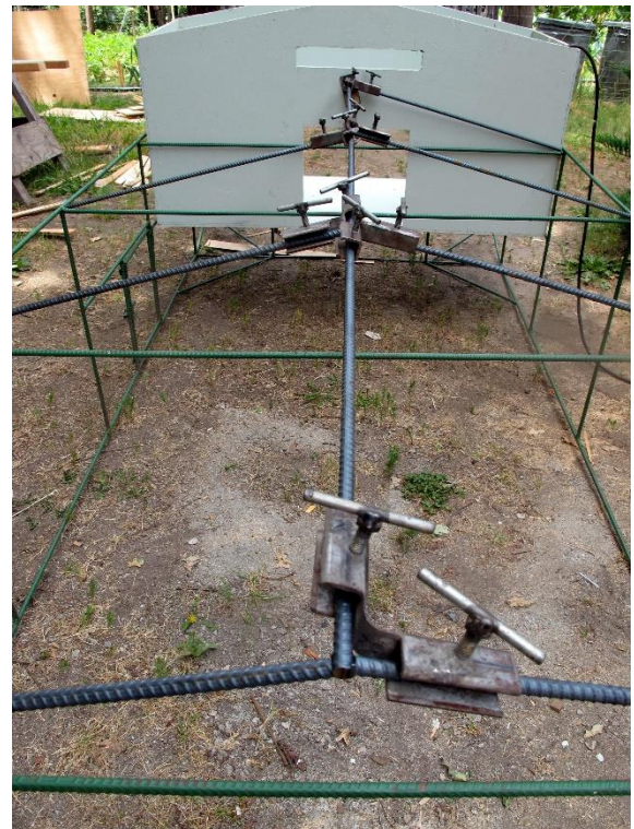
8. Corner clamps fabricated by Wilson to hold rebar in place for welding.
